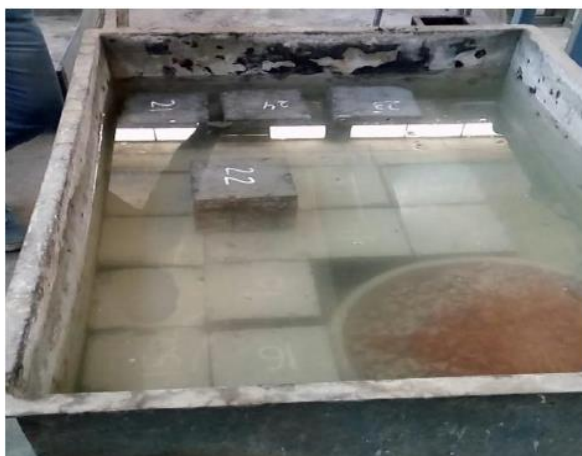
Figure 2: Curing of the casted cube specimens
