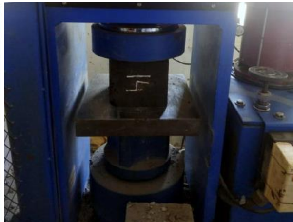
Figure 3: Compressive strength testing using UTM
